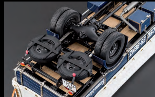
The chassis also features a huge array of fine details such as functional leaf springs and miniaturized brake lines
