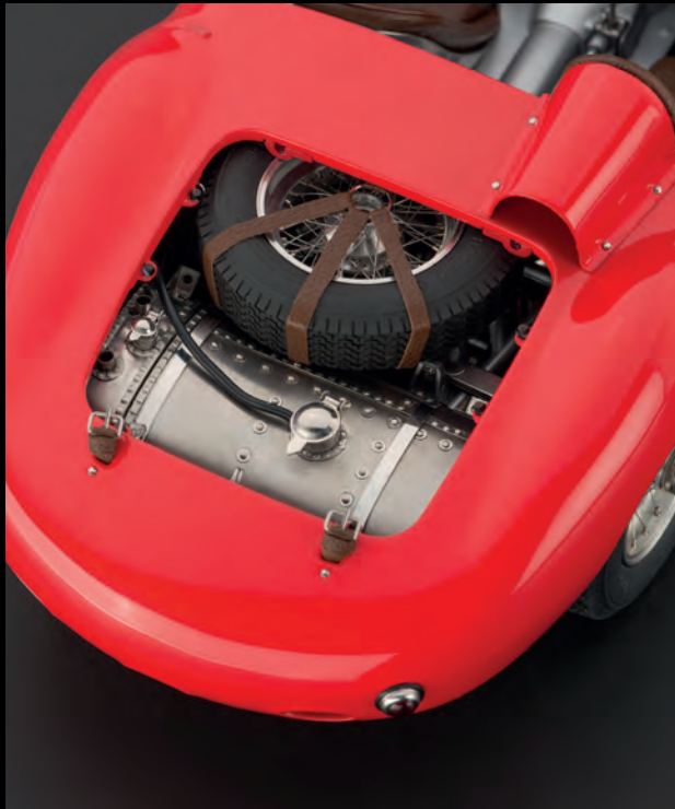
As on the original car, three leather straps tie down the spare wheel in the rear compartment
