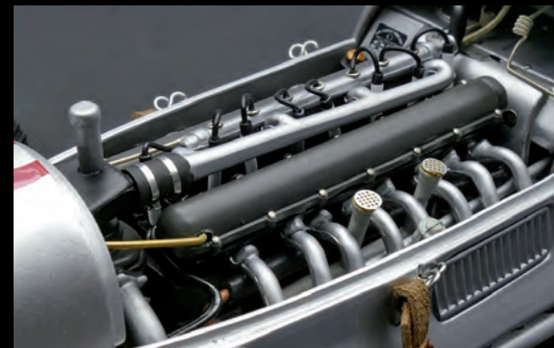
Detailed model replica of the 8-cylinder in-line engine with all ancillaries
