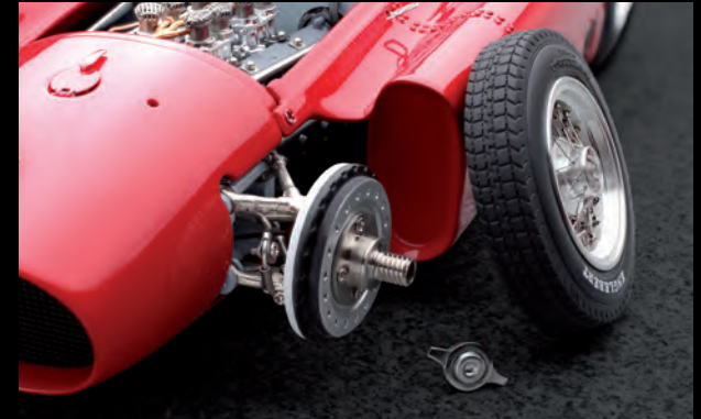
The wishbones of the front wheel suspension are accessible after removing the wheel
