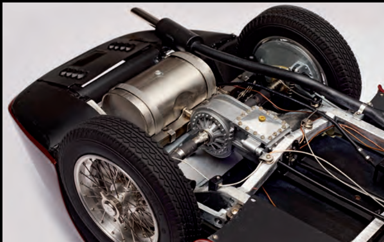
True to the original, the transaxle design combines the gearbox and rear-axle final drive in one unit
