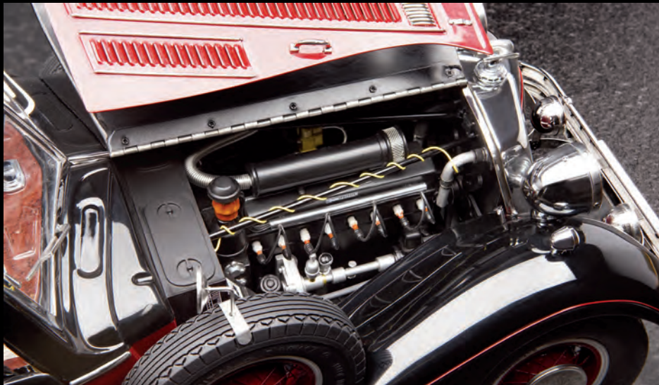
Detailed miniature version of the straight-eight engine with all ancillaries and full wiring
