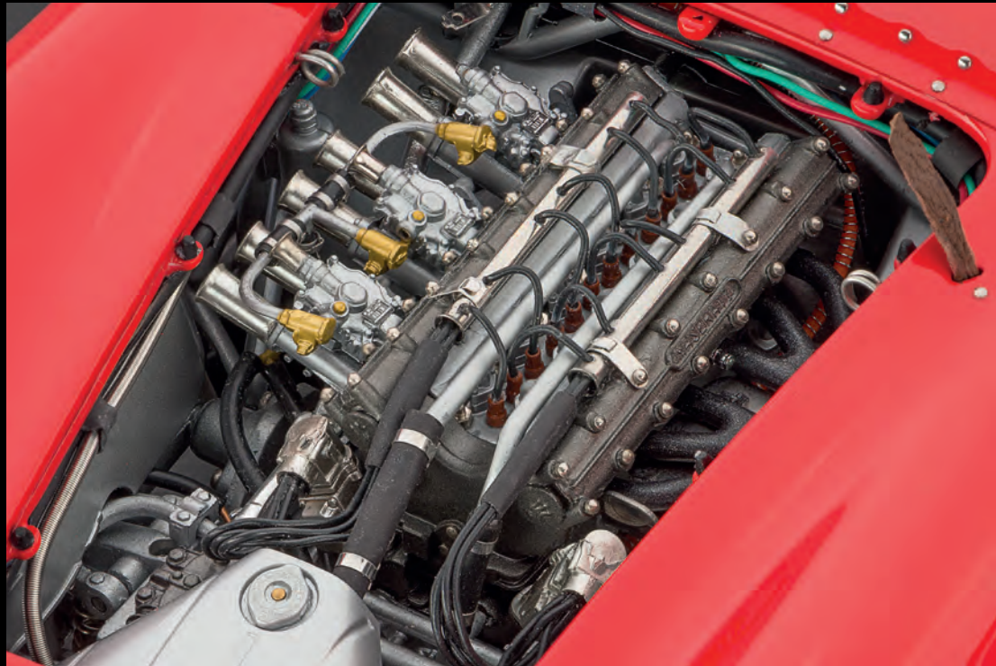
The heart of the race car: a detailed replica of the potent 6-cylinder in-line engine with full wiring and plumbing
