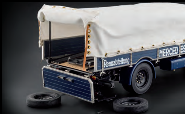
Functional hinged side boards and tail gate, removable tarpaulin held in place by scale-correct leather straps
