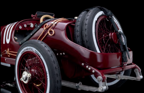
The two-litre race cars were fitted with outboard-mounted spare wheels for long-distance races
