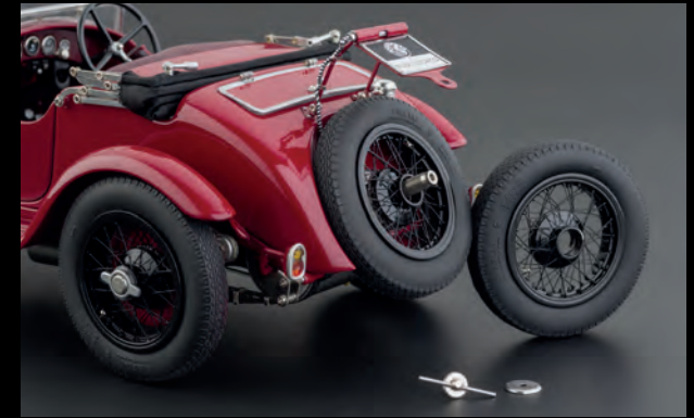
Both spare wheels can be taken off after releasing a T-screw
