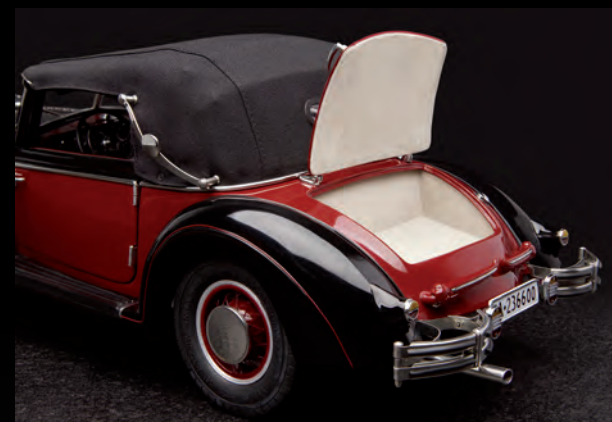
Carpeted boot and passenger compartment, bumpers with rubber pads, as in the original
