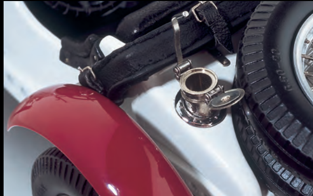
Fully functional petrol tank filler neck
