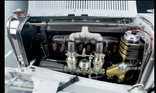
According to test bench trials, the larger of the two competition superchargers (nicknamed the „elephant“ in-house) raised engine output to 310hp
