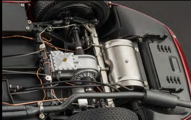
The transaxle design integrates the gearbox and rear-axle final drive in one unit
