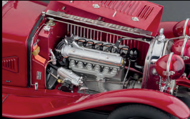
Highly detailed six-cylinder engine with front- mounted Roots supercharger and ancillaries complete with wiring and plumbing
