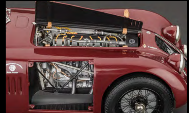
Highly detailed 8-cylinder in-line engine, crankcase with two light-alloy blocks housing with 4 cylinders each
