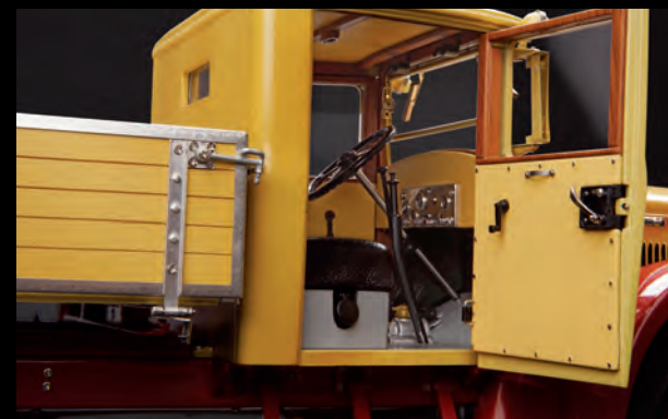
Highly detailed cab with all controls and removable seat bench with leather upholstery
