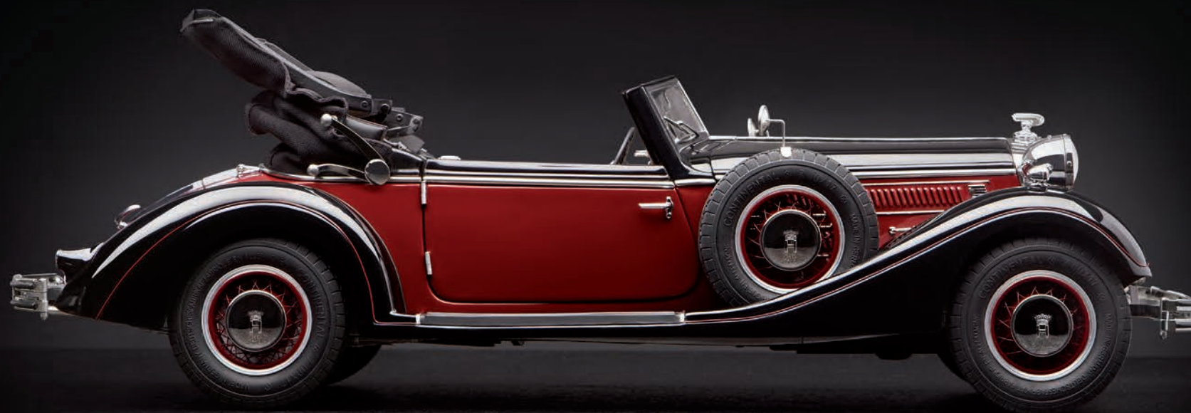
The folding soft top with its accurately re-created metal hinge assembly is fully functional
