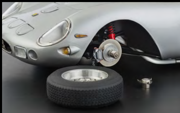
Removable wheels (3-wing central knockoff nut)
