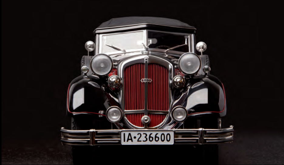
Radiator grille with hand-fitted vertical bars made entirely from stainless steel
