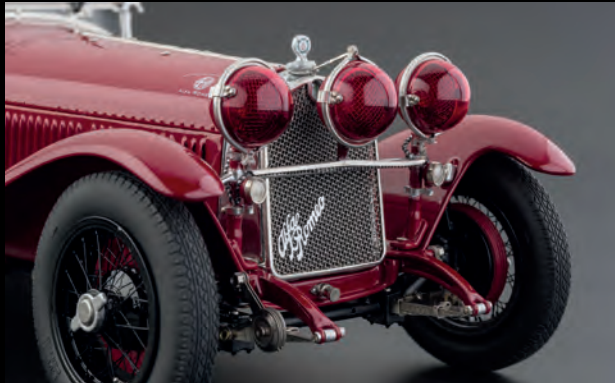
The translucent red headlight covers can be removed – they were intended to improve the aerodynamics of the original car
