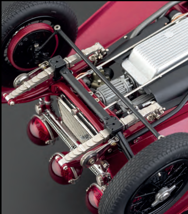
The accurately detailed floor pan is built up from finely finished zinc alloy casting
