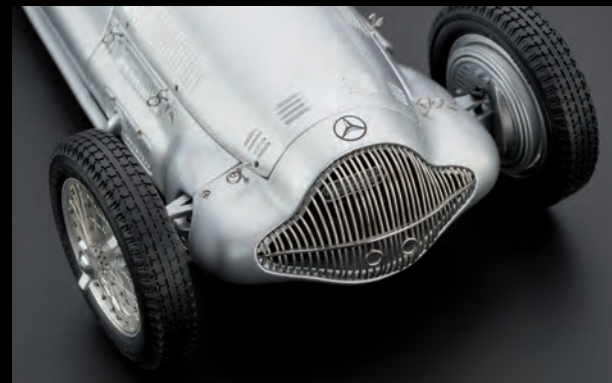
The radiator grille consists of fine, hand-formed and individually soldered wire bars
