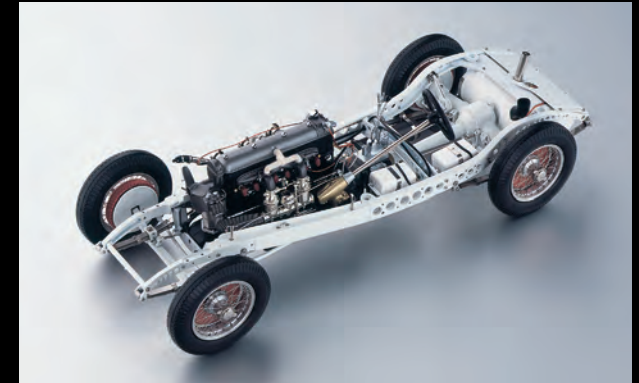
An outstanding feature: the frame members drilled for lightness
