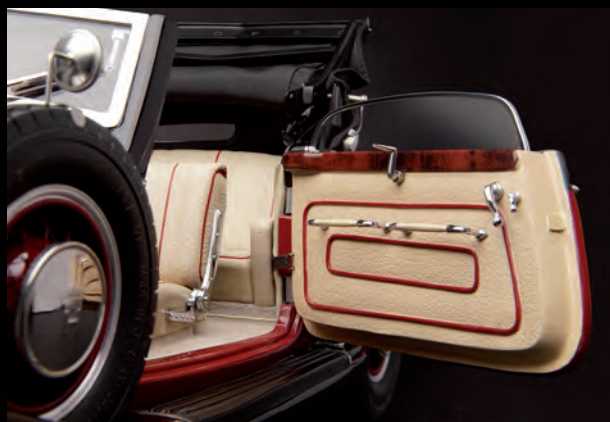
The doors pivot on metal hinges, the side windows can be cranked up and down
