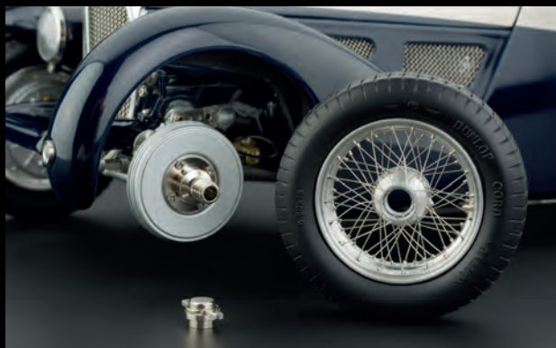
Intricately-spoked wheels and central knock-off nuts with side-dependent right-/left-hand threads
