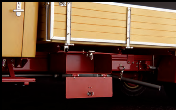
Hinged tool boxes, secured with accurately reproduced and functional locking tabs
