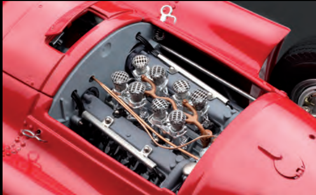
The V8 engine with the cylinders set at a 90° angle is reproduced with maximum detailing
