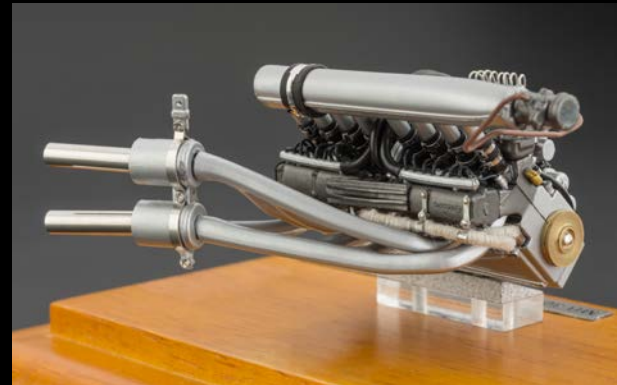
A typical characteristic of the 300 SLR engine are the sidewise installed double exhaust pipes with the small exhaust silencers.
