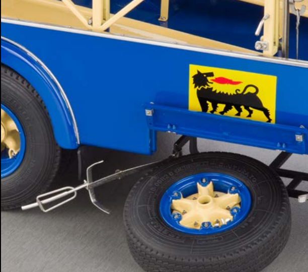
Removable spare wheel with a functional spring clip-lock. Authentic replication of the Trilex wheel assemblage.
