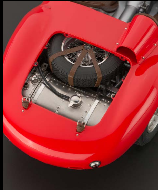
The spare wheel is fastened with three leather straps, as in the original vehicle.
