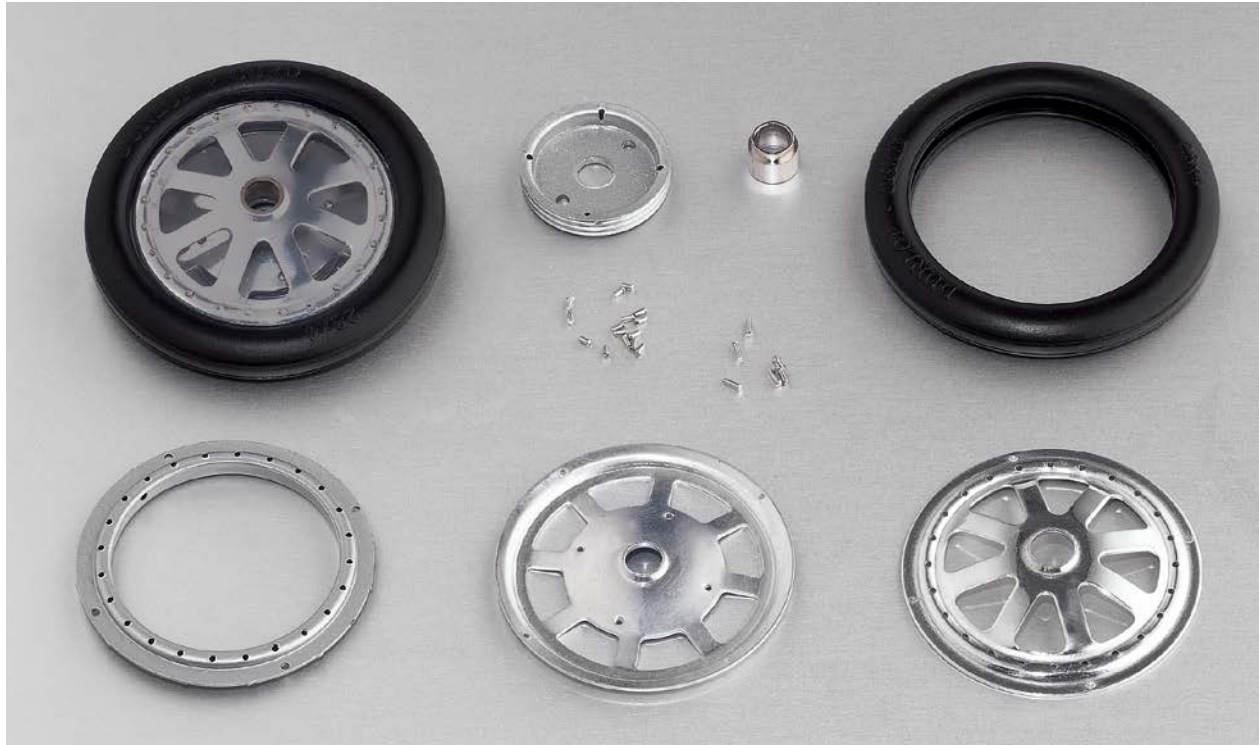
Each wheel is assembled from 35 single parts. With a rim-spoke assemblage akin to the original cast design, the wheel is removable with an authentic quad-winged nut. It also forms a unitary whole with the ripped drum brake. Note the cable-operated brake on the rear axle.
