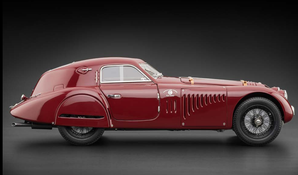
Touring body with a lightweight closed structure (coupé) known as Supperleggera.
