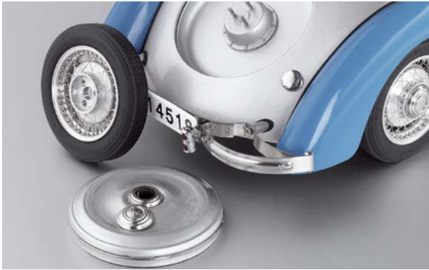
Perfectly spoked wheels with aluminium rims, stainless steel spokes and nipples, all mounted by the hand.
