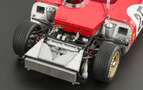
Removable front with screw fixation. Authentically replicated Firestone tires from real rubber.
