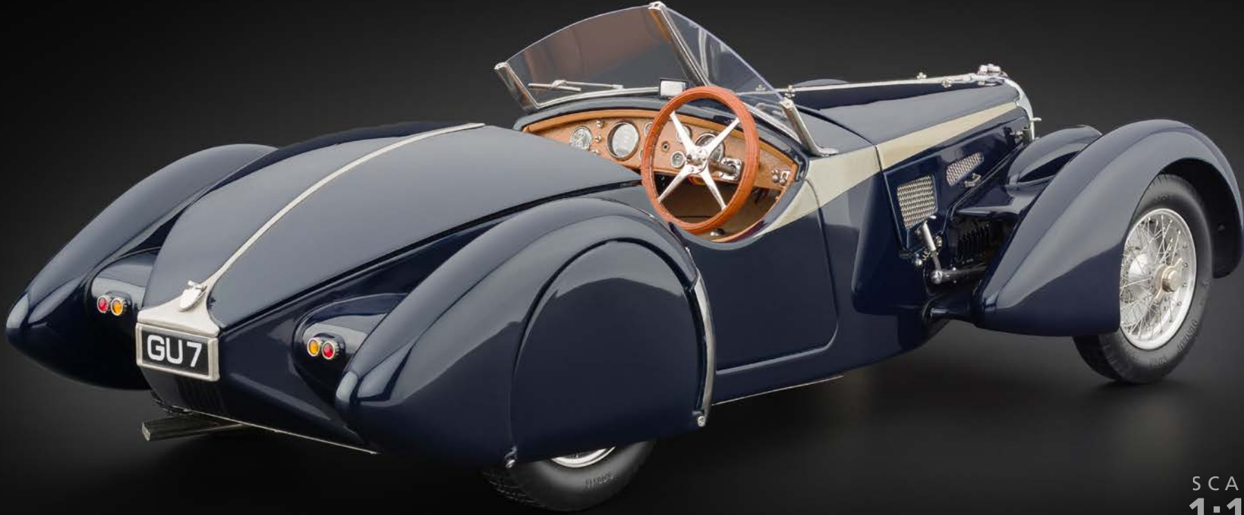
Perfectly spoked wheels and two-wing central locking nuts with right- or left-hand thread for the release of the wheels.
