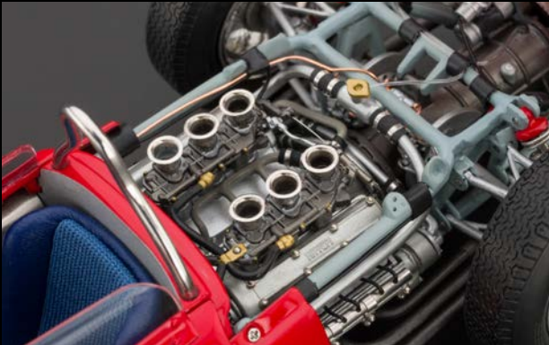
Highly-detailed reconstruction of the six-cylinder V-engine, including gearbox and clutch.
