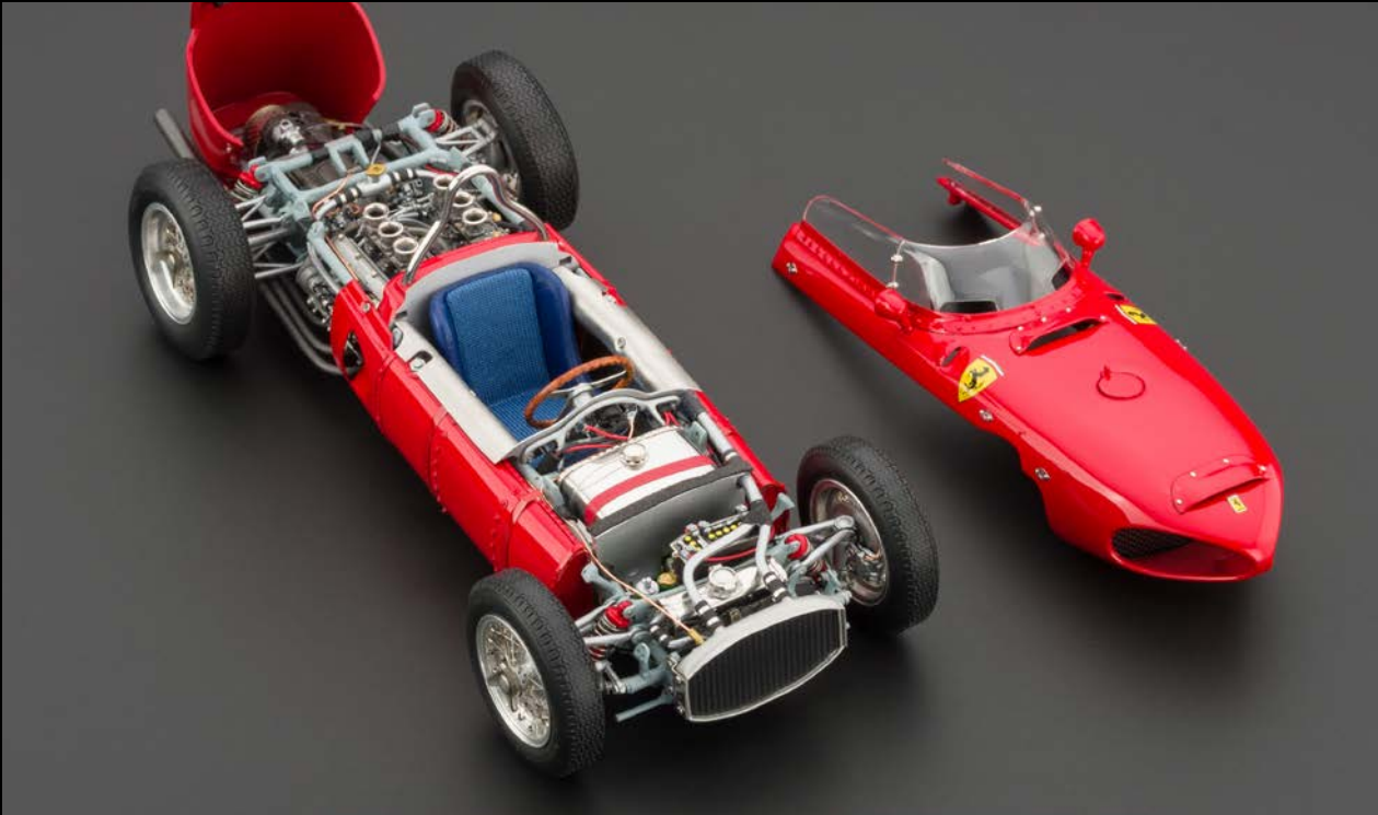
Remove the two screws, and the front part will come off. The oil tank, the additional fuel tank and the painted side fuel tanks are made of stainless steel. Movable tank flap and air inlet for the cockpit cooling.
