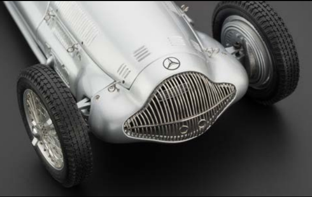
Radiator grill made from fine metal bars soldered by hand.
