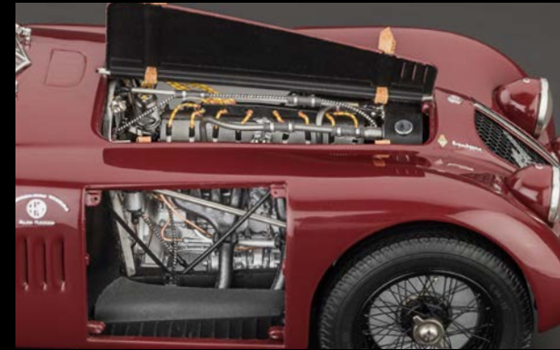
Highly detailed 8-cylinder in-line-engine with crankcase made of two light-metal blocks, each with 4 cylinders.
