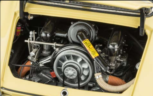
Highly detailed six-cylinder boxer engine, complete with all pipes and cabling.
