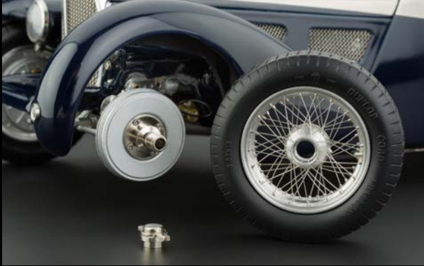
Perfectly spoked wheels and two-wing central locking nuts with right- or left-hand thread for the release of the wheels.
