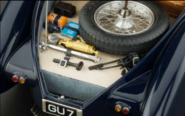
Trunk with enclosed miniature version of the car jack, air-pump, grease gun and toolkit.
