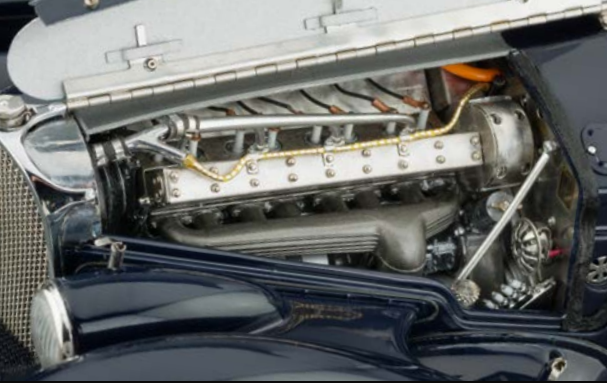
Highly detailed 8-cylinder in-line engine with all aggregates, pipes, and cabling.
