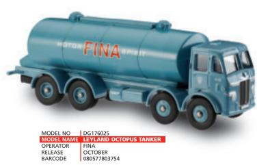
Leyland's post-war '600 Series' range appeared in 1947, the Octopus being the largest model at 22 tons gross vehicle weight. Its plain but tasteful styling still had echoes of wartime austerity. Power unit was Leyland's own 125bhp, 600cu.in diesel.
