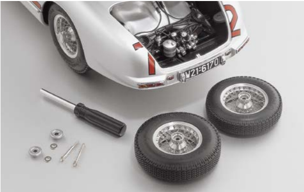
Spoked-wheels on aluminium rims. Each stainless-steel spoke is mounted with a nipple.
