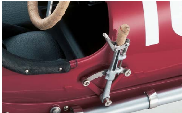
Movable handbreak with a functional catching mechanism and a leather-wrapped grip.
