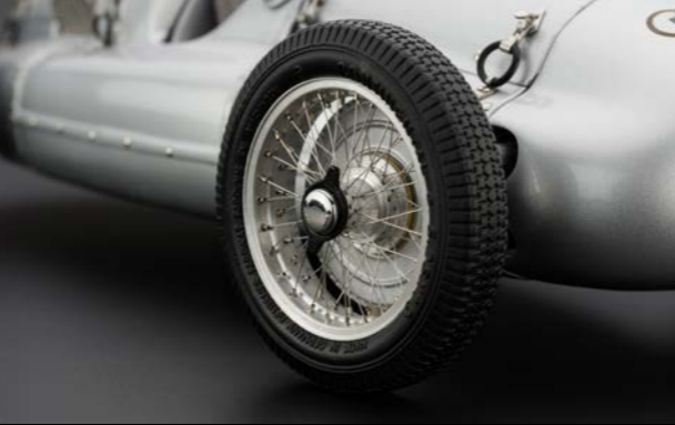
Spoked wheels are each wired with 30 stainless steel spokes.
