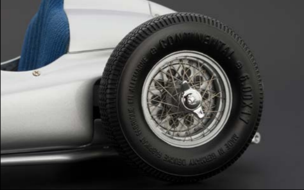
Wheels with hand-assembled spokes. Each has 30 steel spokes individually wired by hand.
