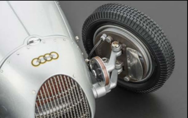
Exact replication of the front friction shock absorber. Brake drums ventilated with metal scoops.
