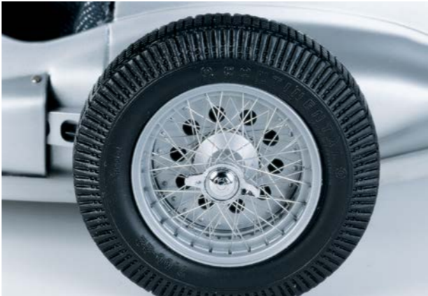
Wheel with filigree spokes. Steel spokes are wired by hand. Authentic-looking tyres.
