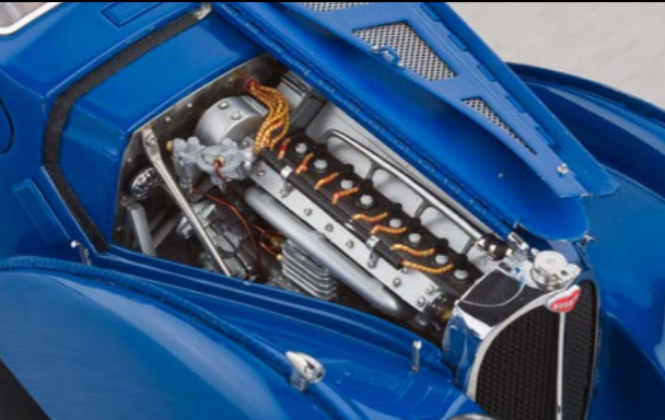
The double leaves of the engine hood each have a hinged side. The 8-cylinder in-line-engine includes all aggregates.
