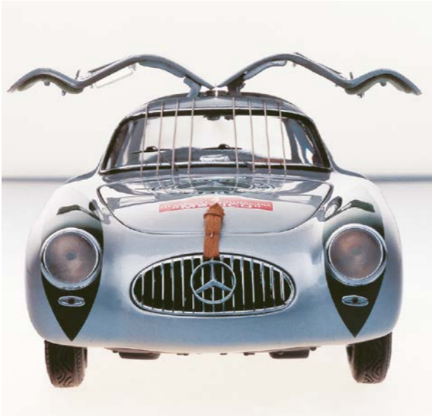
Hand drawn steel bars in front of the windshield, endparts are photo-etched.
