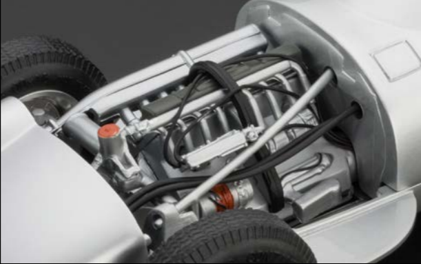
8-cylinder in-line-engine, brakes enclosed. Double exhaust pipes and rear-starter.
