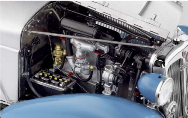
Six-cylinder in-line-engine with all aggregates, cabeling and pipes.
