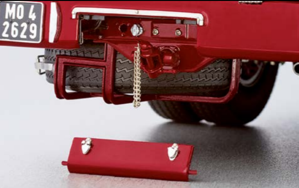
Behind the removable cover is a flanged towing hitch.
