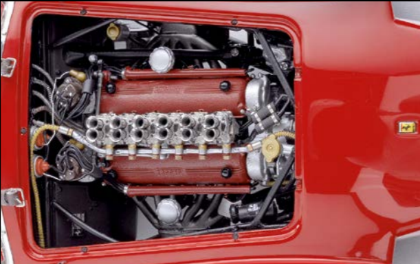
Twelve cylinder V-engine complete with all aggregates, pipes and cabling.
