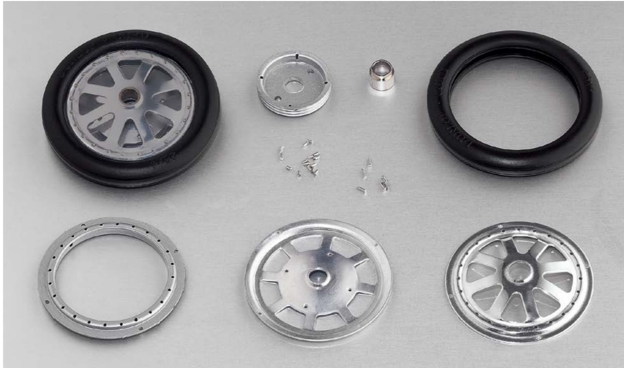
Each wheel is assembled from 35 single parts. With a rim-spoke assemblage akin to the original cast design, the wheel is removable with an authentic quad-winged nut. It also forms a unitary whole with the ripped drum brake. Note the cable-operated brake on the rear axle.
