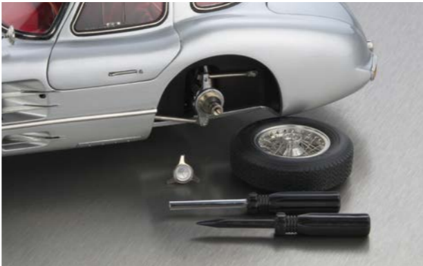
Removable three-wing central locking nuts. The central locking nuts are so designed that they are side-specific.
