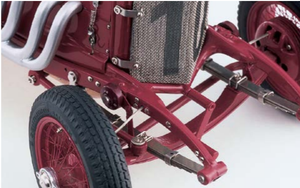
Functional multi-layer compound springs (6 lays) on the front and rear axle.
