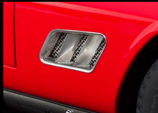
The side engine ventilators are equipped with ventilation fins of stainless steel against a meshed wire of metal.
