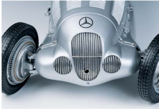
Radiator grill is made by soldering 35 stainless steel bars and mounted in place against a fine metal mesh.
