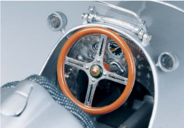
Instrument panel of stainless steel, polished in a brush finish that features a pattern of marbles.
