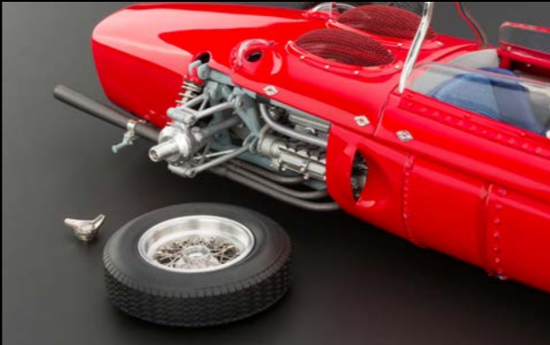
Removable wheels on aluminium rims and stainless steel spokes with nipples.
