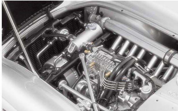
Highly detailed 8-cylinder in-line-engine installed in angular position and complete with all pipes and cabling.
