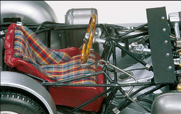
Cockpit seat covered in textile fabric with a leather headrest. Precisely replicated tubular space frame with metal bars.
