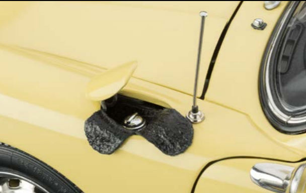
Tank top that flaps open to reveal leather cloth (scratch protection). Retractable antenna.
