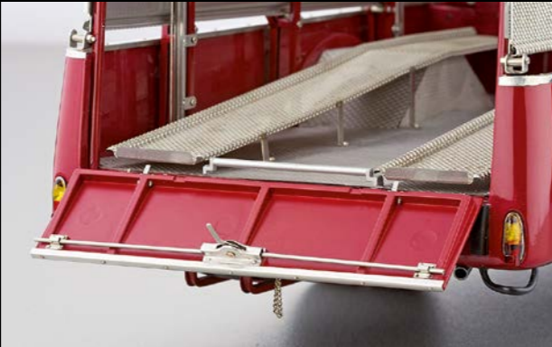
The tailgate is equipped with a functional bar-slide locking mechanism.
