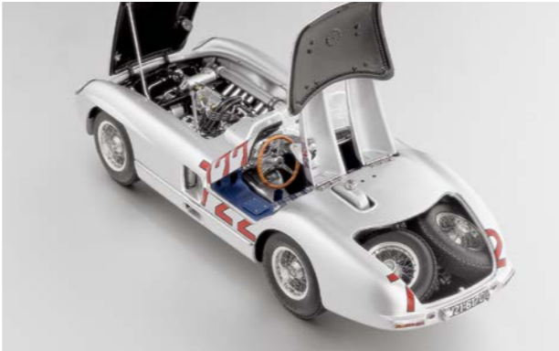
The headrest dome is a part of the hatch, which opens to allow access to the spare wheels.
