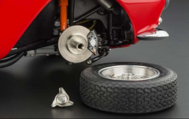
Screwable Borrani wheel nut enables you to remove the wheel.
