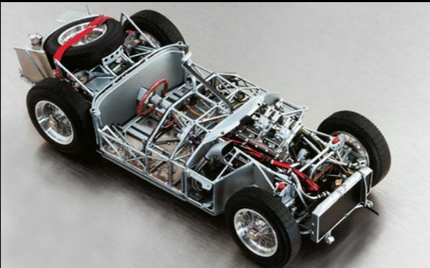
The innovative frame reconstructed true to the original and made from filigrane metal tubes.
