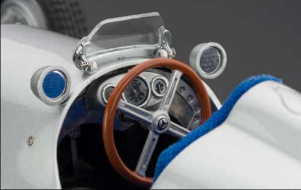
Stainless steel panel polished to a brush finish featuring a pattern of marbles and assembled with instruments by hand.
