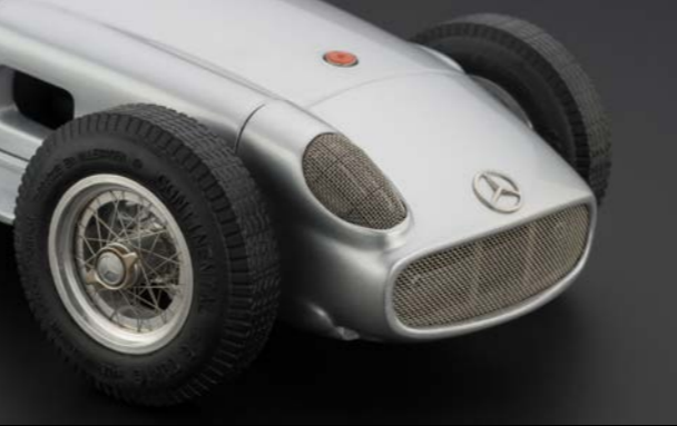
Wheels with hand-assembled spokes. Air-inlet cover and radiator grille made of stainless steel mesh.
