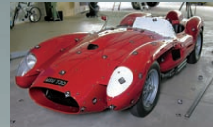
■ Marks on a car that support the digitalization of the body.
