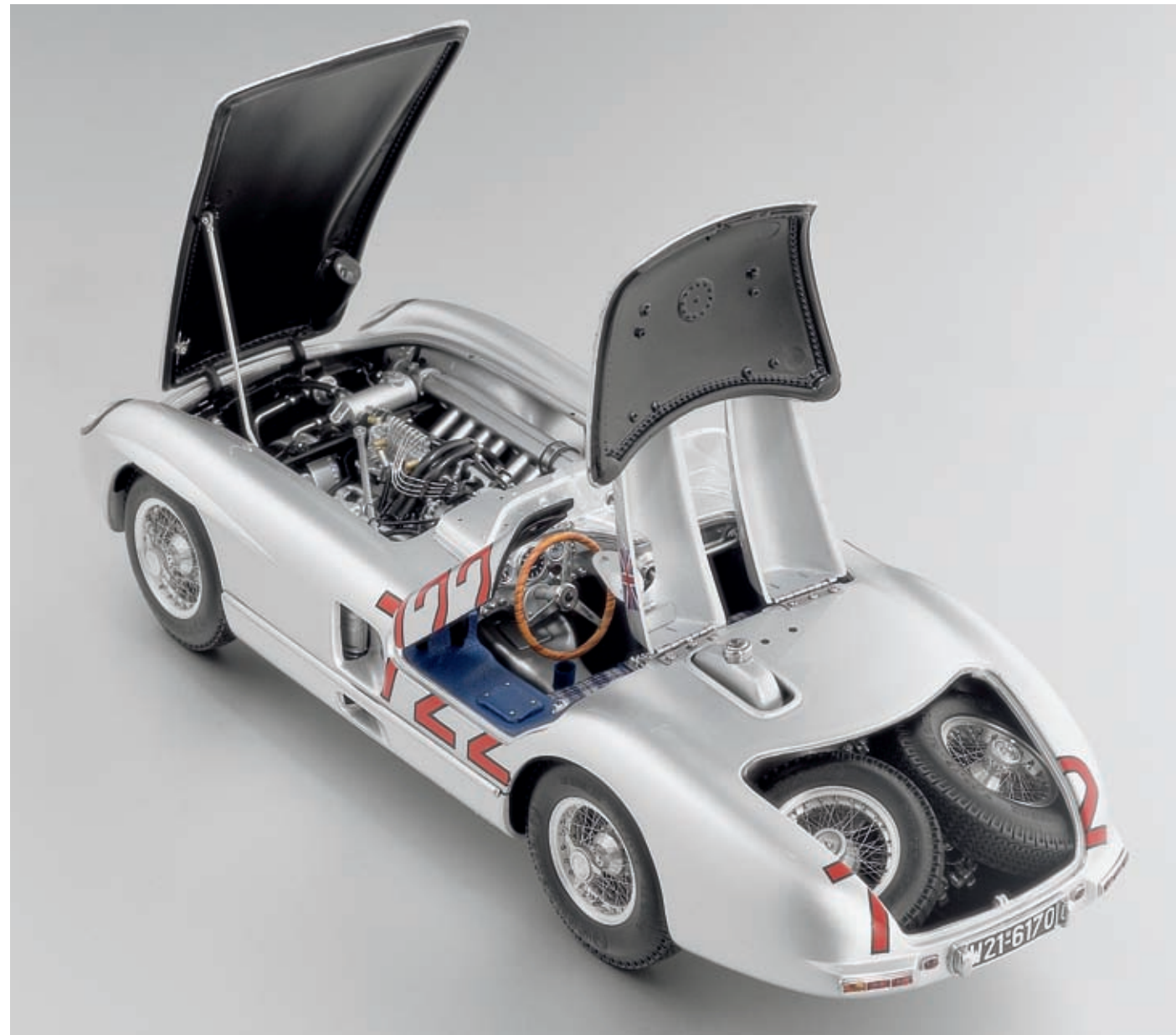
■ The headrest dome connects with the hatch. It can be flipped up as one single unit to gain access to the spare wheels. The engine hood has a tent prop
