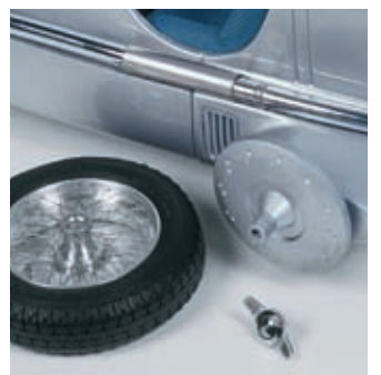
■ Wheel hub and rim are of milled aluminium ■ 140 drilled holes of 0,4 mm diameter in hub and rim for the insertion of the spokes ■ Each wheel is hand assembled from 70 spokes of 0,2 mm diameter stainless steel wire ■ Mounting and dismounting of the wheels is possible with the double winged central locking nut with fine thread screw
