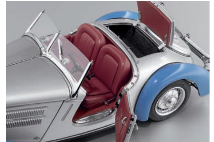
■ Windshield with high gloss chromed metal frame and installed wiper motors ■ Doors and trunk deck are covered with leather at the inside
