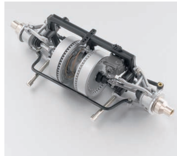
■ Front wheel suspension with inside drum brakes
