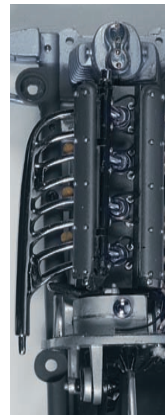
■ Exhaust manifold of metal with highly polished chrom finish
