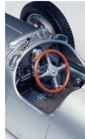
■ Costly dashboard ■ Sides with metal covering ■ Cockpit-seat with real textile and head rest with real leather covering
