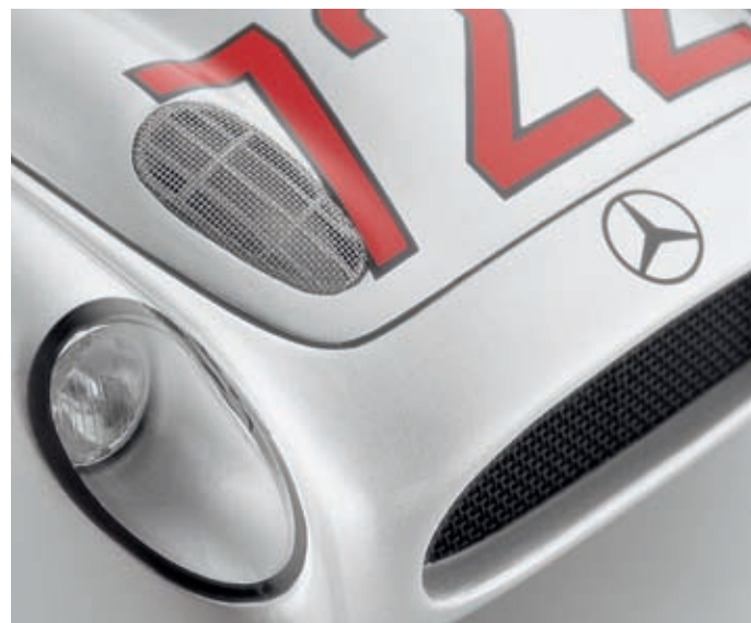
■ The front-right engine hood fitted with a filigree grill for the cooler and engine air-inlet duct
