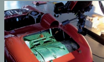
■ Scanning the body of an original vehicle with the help of a special camera.
