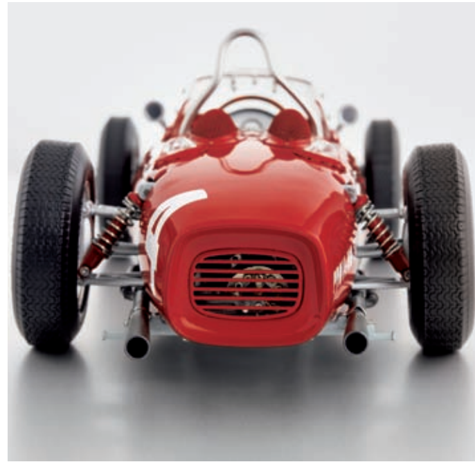
■ Pure dynamic! Negative camber at the rear wheels, just like the original car. Behind the rear-end fence, you can identify the exterior clutch.
