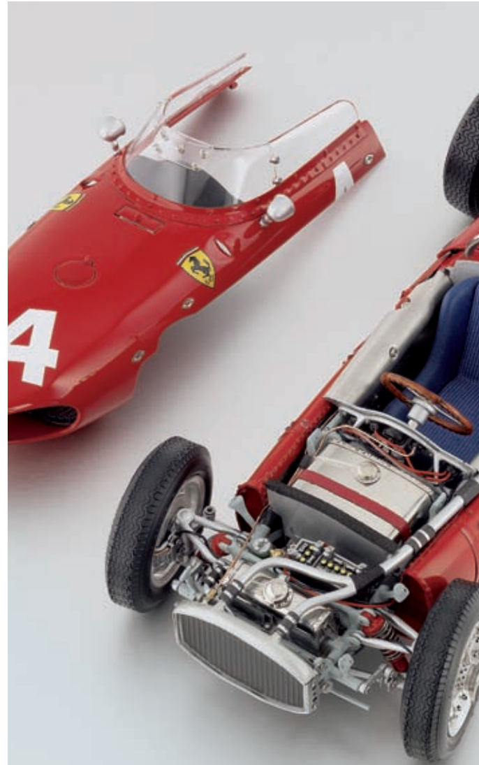
■ Remove the two screws, and the front part will come off ■ The oil tank, the additional fuel tank and the painted side fuel tanks are made of stainless steel ■ Movable tank flap and air inlet for the cockpit cooling
