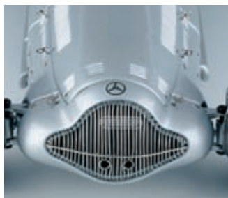
■ Radiator grill made of fine, hand-drawn wires, soldered individually
