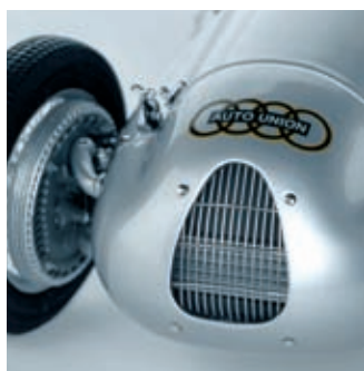
■ Radiator grill consisting of 16 pieces of steel wires soldered individually by hand
