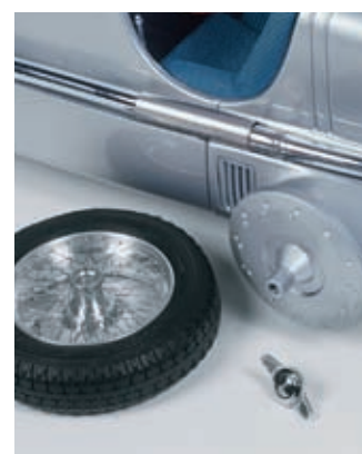
■ Wheel hub and rim are of milled aluminium ■ 140 drilled holes of 0,4 mm diameter in hub and rim for the insertion of the spokes ■ Each wheel is hand assembled from 70 spokes of 0,2 mm diameter stainless steel wire ■ Mounting and dismounting of the wheels is possible with the double winged central locking nut with fine thread screw
