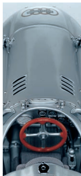
■ The engine hood fastening consists of 32 parts ■ Driver's seat covered with textile
