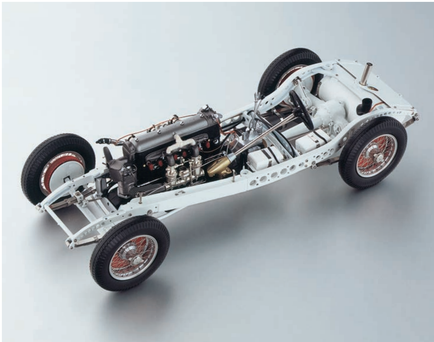
■ Authentic replication of the weight-reduced steel frame and its exact hole pattern.
