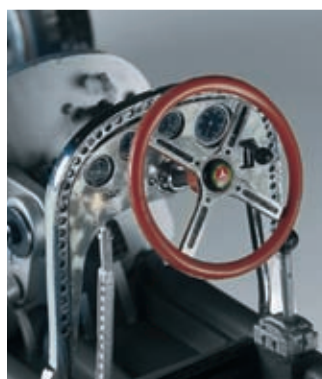
■ Instrument panel of stainless steel with a marbled surface and hand inserted instruments
