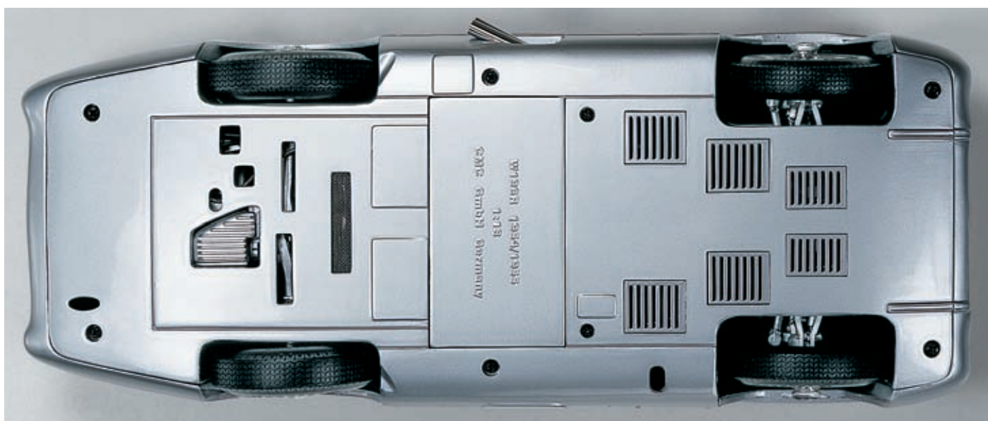
■ By unscrewing of six little screws at the floor panel, the complete body can be removed. This enables a good view at the insight to the tubular space frame as well as chassis and power train.
