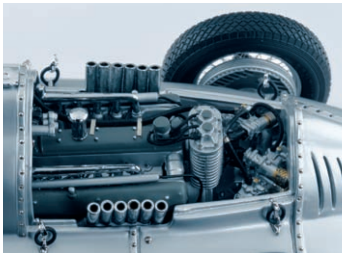
■ True to the original displayed 12-cylinder-engine ■ 12 exhaust pipes made of metal
