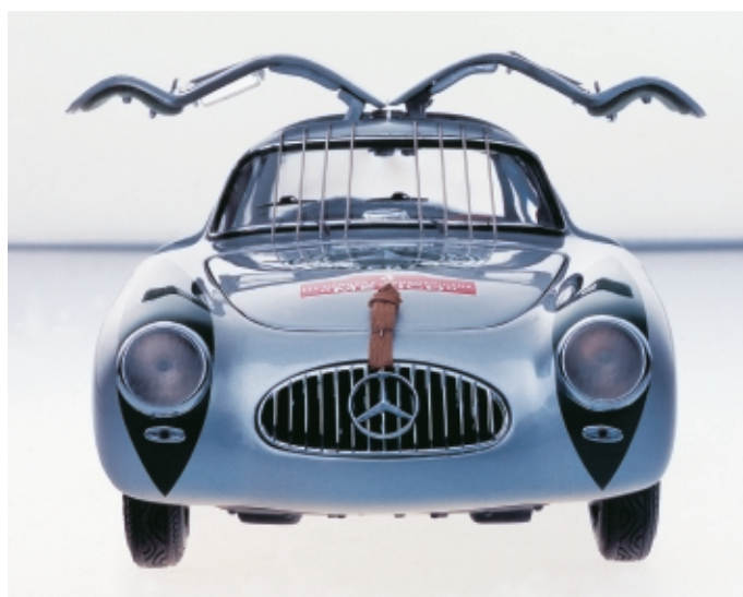
■ Hand drawn steel bars in front of the windshield, endparts are photo-etched
