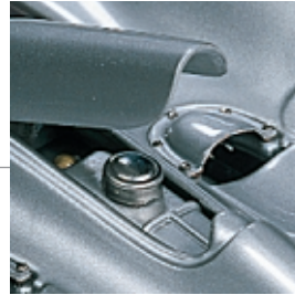
Sheet copper formed and with metal rivets fixed air outlet hoods. Movable fuel tank cap.
