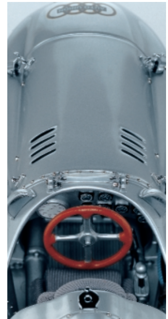
■ The engine hood fastening consists of 32 parts ■ Driver's seat covered with textile
