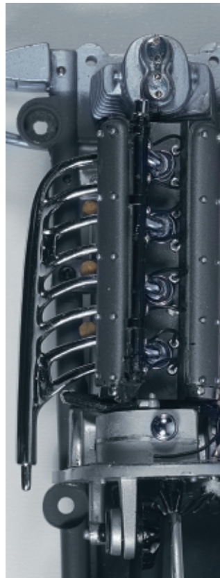
■ Exhaust manifold of metal with highly polished chrom finish
