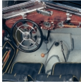
The dash board of the Horch 853: hand implemented round instruments with sharply outlined scales, many operating units and switches.
