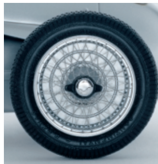
■ Spoke wheels consisting each of 30 hand assembled steel wires
