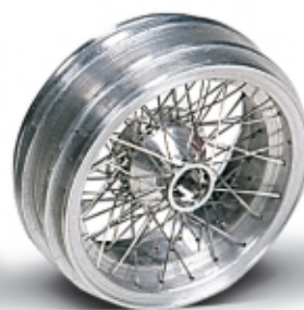
Wheels of the W 196 R Streamliner. Mounting and dismounting of the wheels is possible with the double winged central locking nut with fine thread screw. Each wheel includes 72 single spokes on three different levels.
