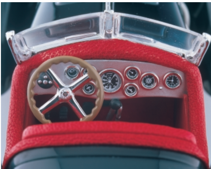
■ Interior with very detailed dashboard and perfect finish: seats, framing of the cockpits outer edge and hoodbelts are of real leather
