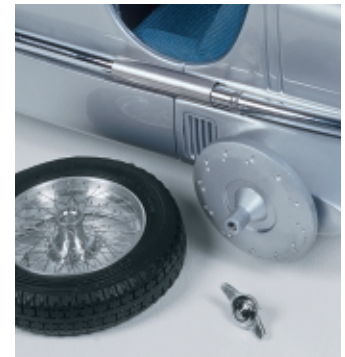
■ Wheel hub and rim are of milled aluminium ■ 140 drilled holes of 0,4 mm diameter in hub and rim for the insertion of the spokes ■ Each wheel is hand assembled from 70 spokes of 0,2 mm diameter stainless steel wire ■ Mounting and dismounting of the wheels is possible with the double winged central locking nut with fine thread screw
