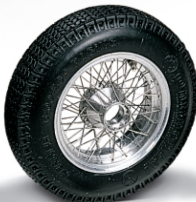
Wheels of the W 196 R Streamliner. Mounting and dismounting of the wheels is possible with the double winged central locking nut with fine thread screw. Each wheel includes 72 single spokes on three different levels.
