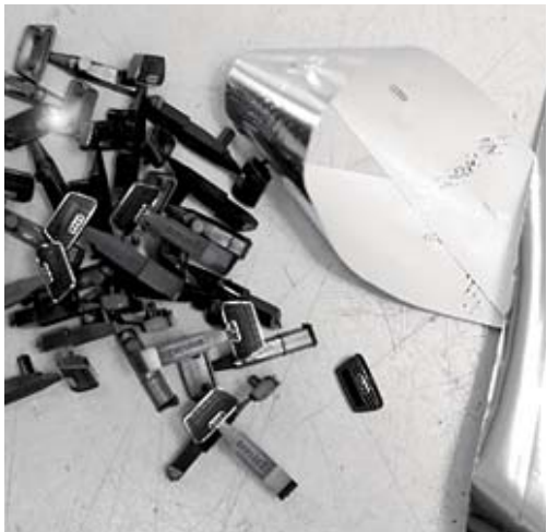
Even the chrome-coloured attachments are reproduced. A chrome layer is thus applied manually to the parts in question.
